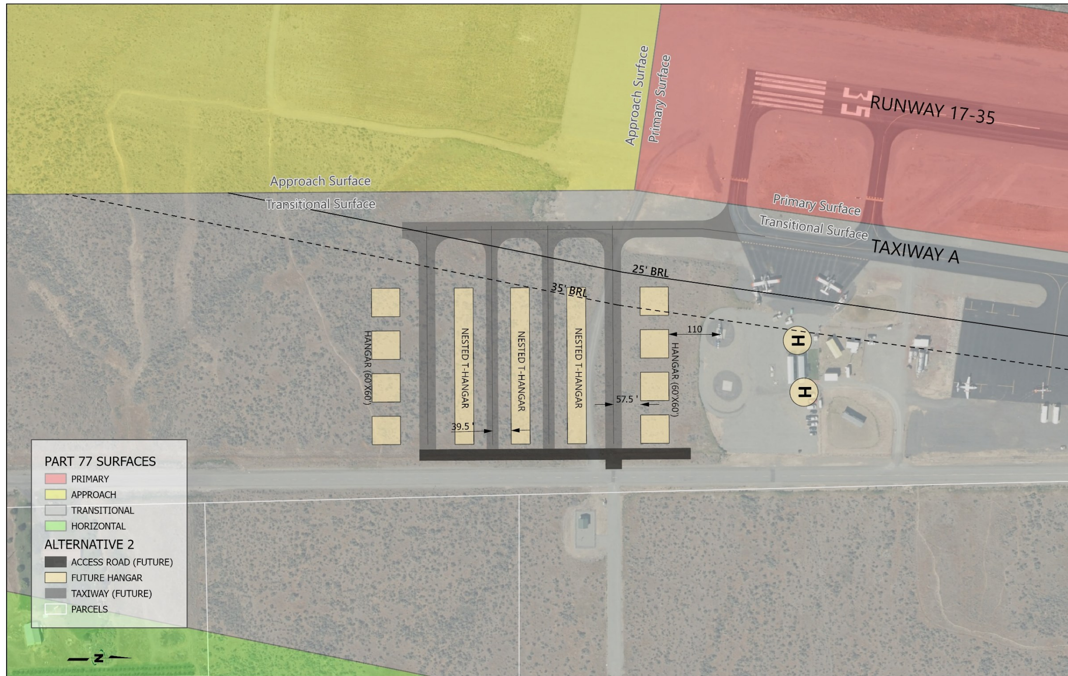
FIGURE 5.2 ALTERNATIVE LANDSIDE CONFIGURATION NO. 2 - HANGAR DEVELOPMENT ON THE SOUTHEAST SIDE OF TAXIWAY A
