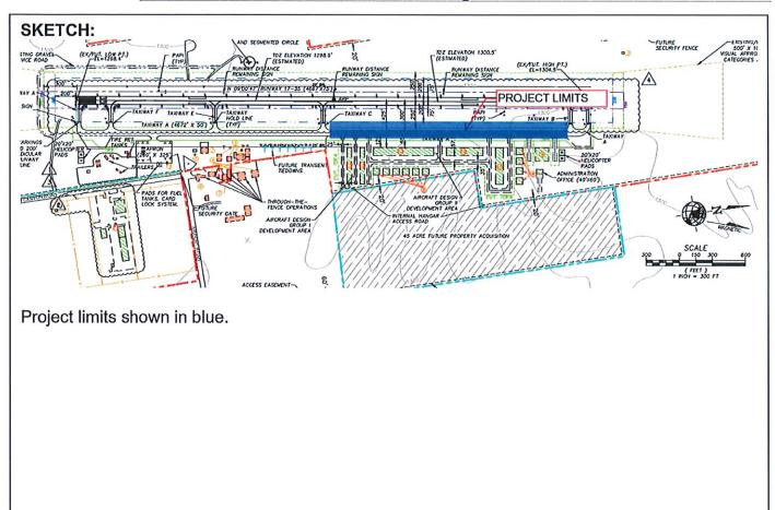
JUSTIFICATION: The north portion of parallel Taxiway A requires reconstruction due to excessive pavement deterioration. The is the design phase of the project. This pavement has a PCI of 37 (2018). In addition to the replacement of the taxiway, the adjacent area will be graded to match any changes in finished taxiway grade.
